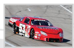
Spears SRL South West Tour Car: "Bad to the Bone"! This fiberglass body, 2,900 Ib car has 570 hp on a short 101" wheelbase. Cole is looking forward to the upcoming season knowing this is the toughest racing on the West Coast.
